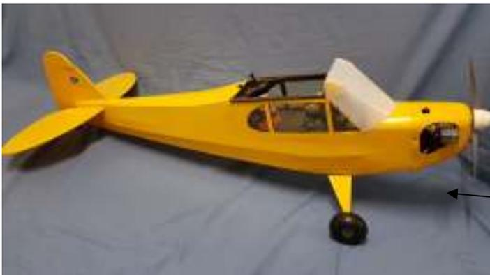
The Thunder Tiger J3 Cub is under reconstruction after a very bad roll in after takeoff. The fuselage is complete and re-covered awaiting it's Cub stripe and some wings.
